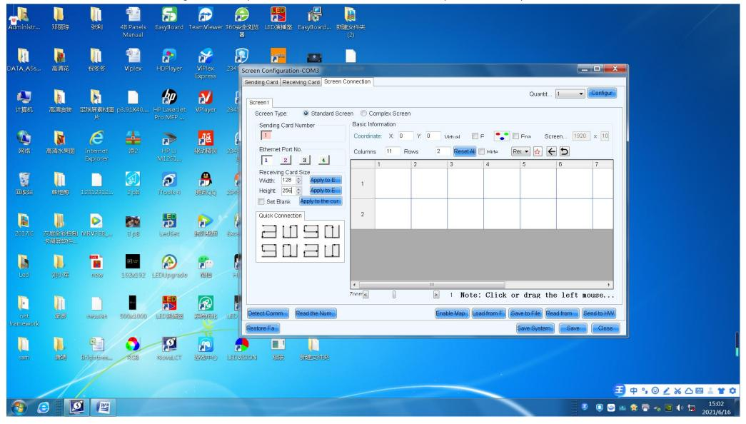
Set the receiving card size at 128x256P. Then make mappings, like it. Remember it is front viewing. After that click sent to HW and save.
