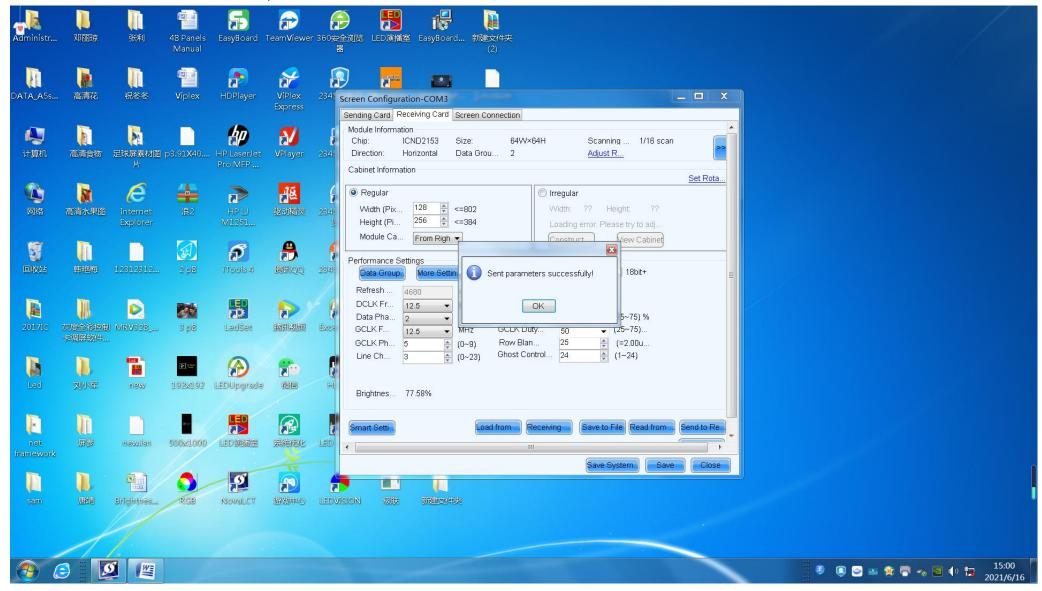
Now move to screen connection. Click configure first. Then you can set columns x rows at 11x2. Just like the panels installation you made.
